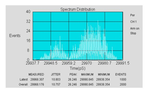
100 MHz (10ns) PLL output. For comparing to CSA 803A, DTS measures time duration from rising edge 1 to rising edge 4 or effectively 3 cycles. As can be seen, the DTS correlates well in rms jitter and shape of the bimodal histograms.
