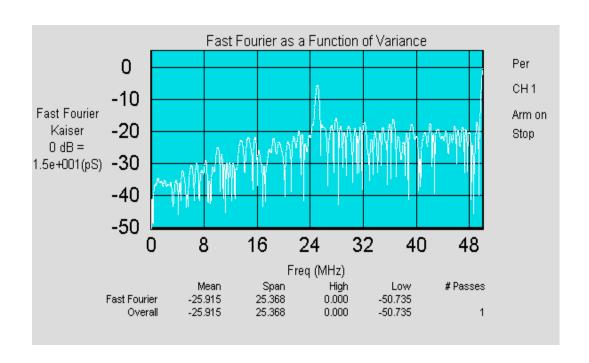
Jitter Analysis FFT of 100MHz PLL output. Modulation detected at 50 and 25 MHz.
