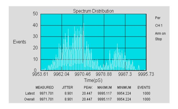
Same signal as above, except DTS is measuring from 1 rising edge to 2nd rising edge (1 cycle or period). Notice lower jitter and shifting of histogram shapes. CSA 803A cannot easily measure just 1 cycle because of minimum delay requirement.
