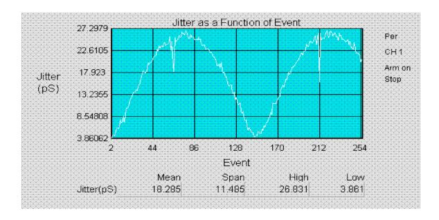
Above is DTS 2070 Jitter Analysis plot for a 19.4 MHz oscillator signal to an ATM device. This modulation is caused by the 130 kHz switching power supply coupling to the test fixture.
