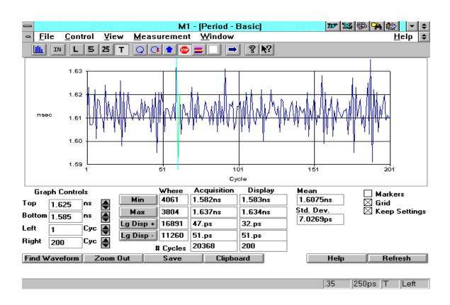
The above is a cycle by cycle plot using a 4 GSa/sec real time digitizer with custom software. You cannot resolve the 20 ps period push out due to the lower resolution of the digitizer.
