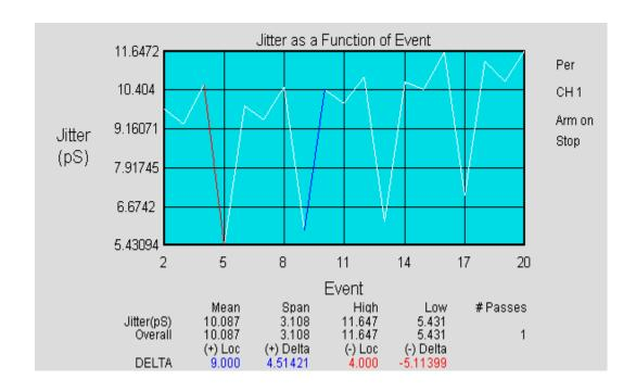
Jitter Analysis of 100 MHz PLL output. Count was set to 20. This is a zoomed plot of the above. Notice the distinct pattern to the accumuated jitter.
