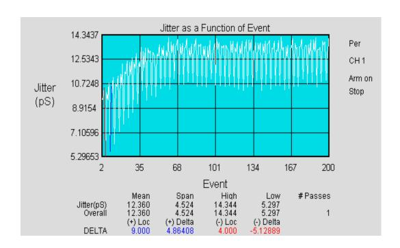
Jitter Analysis of 100 MHz PLL output. Up to count 200. Notice the accumulated jitter modulation in the time domain.
