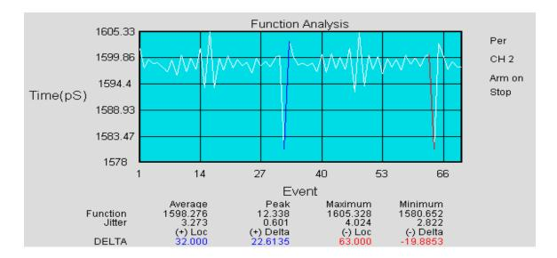
Above is a DTS 2070 Function Analysis plot on a 622 MHz ATM device. Notice the 20 ps short cycle every 32 cycles. The 800 fs resolution of DTS 2070 allows one to "see" the small period push out.
