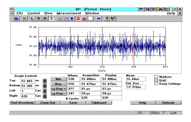
The above plot is a cycle by cycle plot using a 4 GSa/sec real time digitizer with custom post processing software. You cannot see any modulation due to the small record length.
